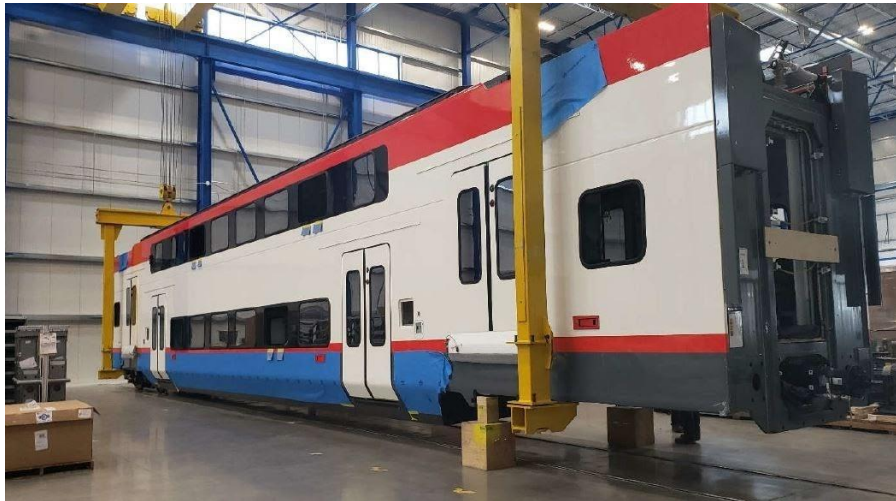
Lifting or lowering one end of the car simulates a vertical curve at the opposite truck.
