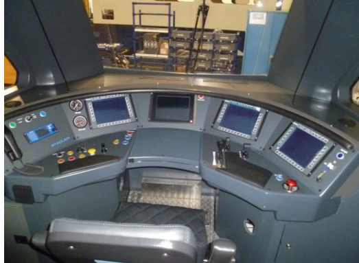
Mockup of engineer's console and seat within the cab
