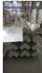
Carbody - Aluminium Section of Roof End Structure
