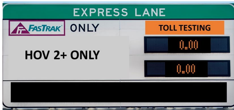
Variable Toll Message Sign
