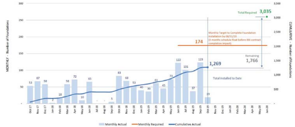
Figure 2-5 OCS Foundation Production
