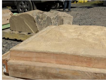
Test Blocks for Tunnel 4 South Portal Archstones
