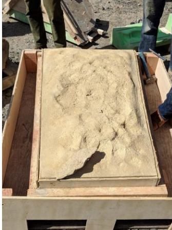
Test Blocks for Tunnel 4 South Portal Archstones
