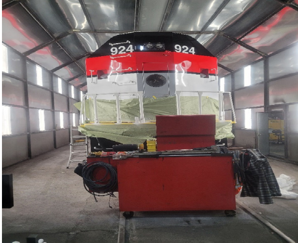
Photo 1 - Locomotive 924 under painting.
