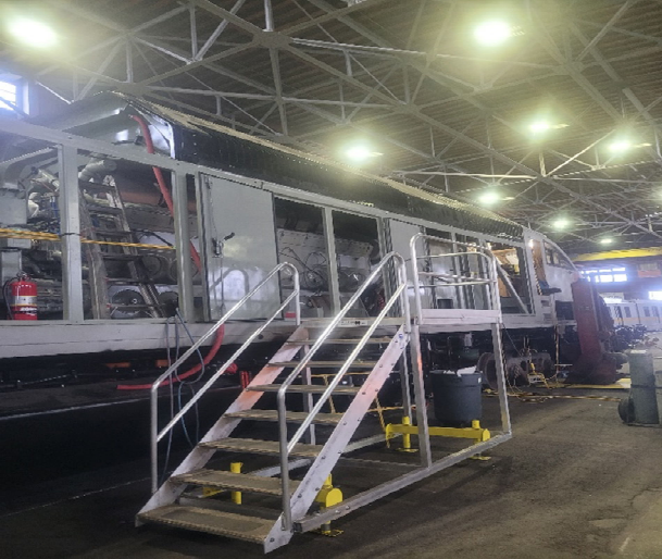
Photo 3 - Locomotive 925 engine installed.
