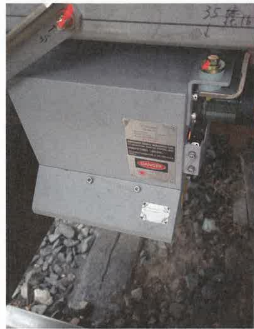
On the left, two workers stand in front of Omaha Track trackwork technology. Top right shows a closer look at one of RailWorks' flash-butt welding trucks. Bottom right features Kawasaki's locomotive mounted autonomous track geometry monitoring device.
