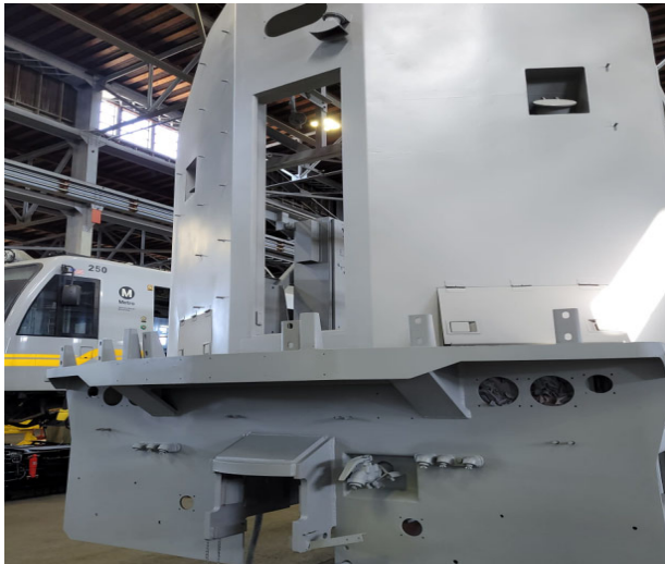
Photo 3 - Locomotive 926 under painting.
