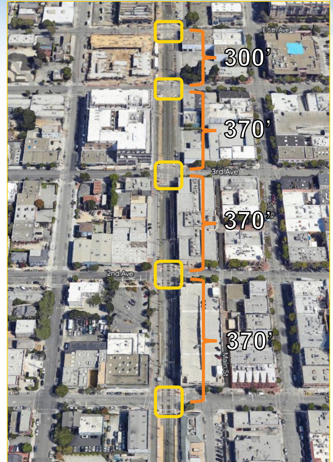
Closely spaced crossings in Downtown San Mateo
