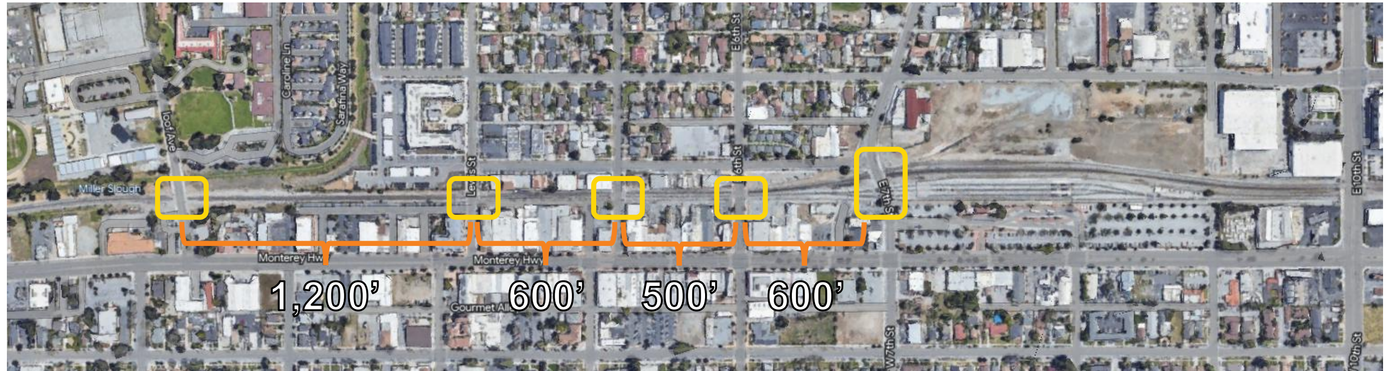
Closely spaced crossings in UPRR ROW in Downtown Gilroy
