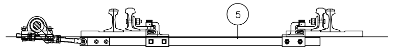
REAR HELPER (ROD NO 4) DRIVE ROD ASSEMBLY REAR HELPER ROD CRANK ATTACHES TO ROD PIN
