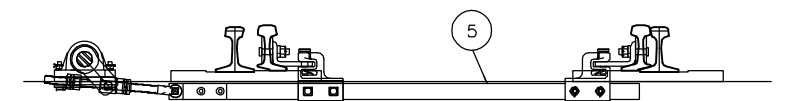
REAR HELPER (ROD NO 4) DRIVE ROD ASSEMBLY REAR HELPER ROD CRANK ATTACHES TO ROD PIN
