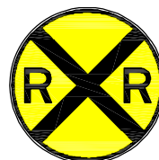
W10-1 HIGHWAY-RAIL GRADE CROSSING ADVANCE WARNING
