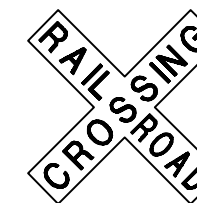
R15-1 RAILROAD CROSSING
