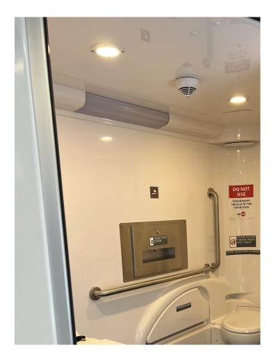
Based on my code and regulatory background and knowledge, and what an accessible bathroom should look like, the picture shown is one of the new "accessible" bathrooms on the new CalTrain cars, but it appears to not be accessible to those using many manual and most electric mobility devices!
