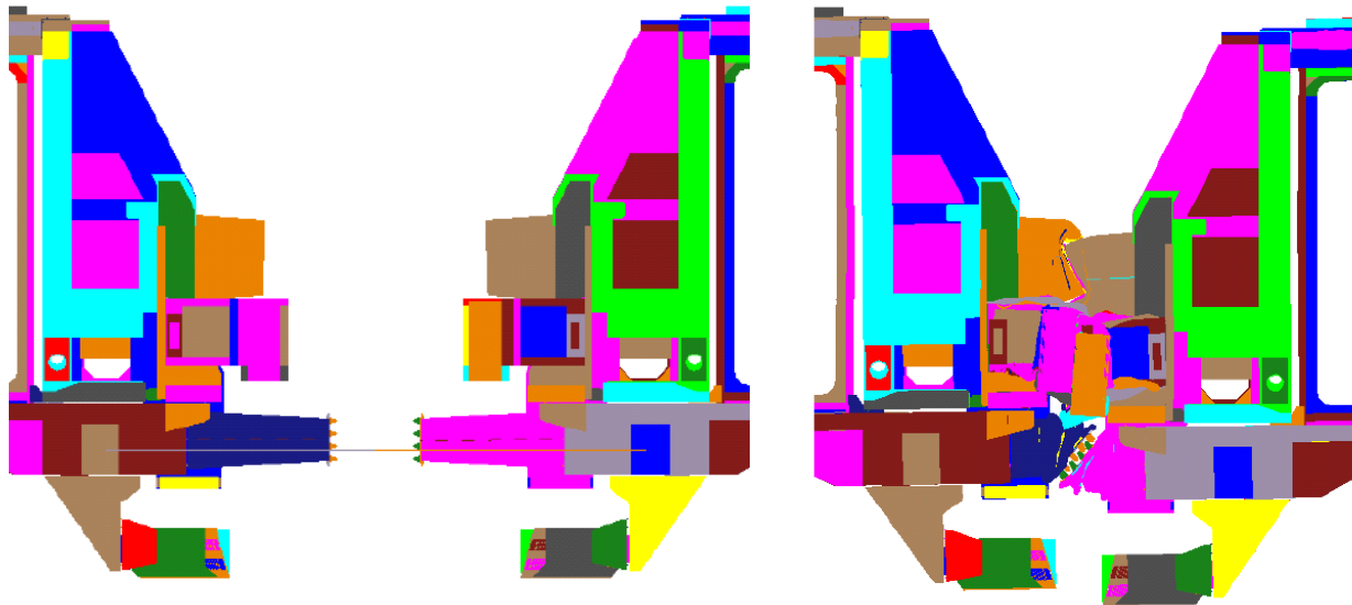
Figure 63 - Pre- and Post-Impact Alstom Trainsets
