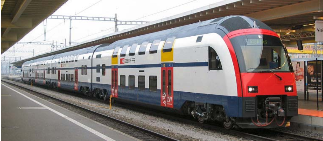
Figure 12 - Siemens Desiro 514 Double Deck EMU Trainset
