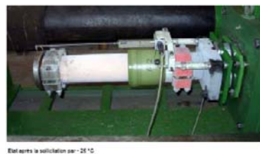
Figure 27 - Intermediate Connection Energy Absorbers (Courtesy Alstom)
