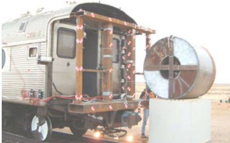
Figure 29 - Steel Coil Impact Test Setup
