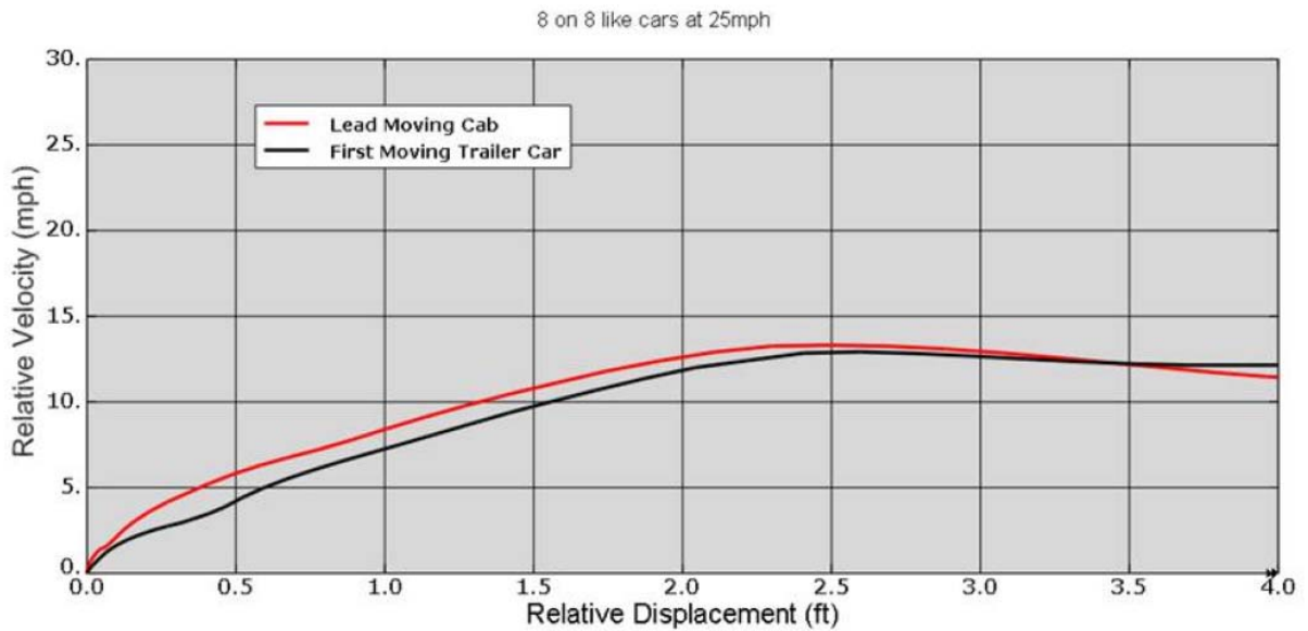
Figure 65 - 8-Car 25 mph Like Train Impact Secondary Impact Velocity
