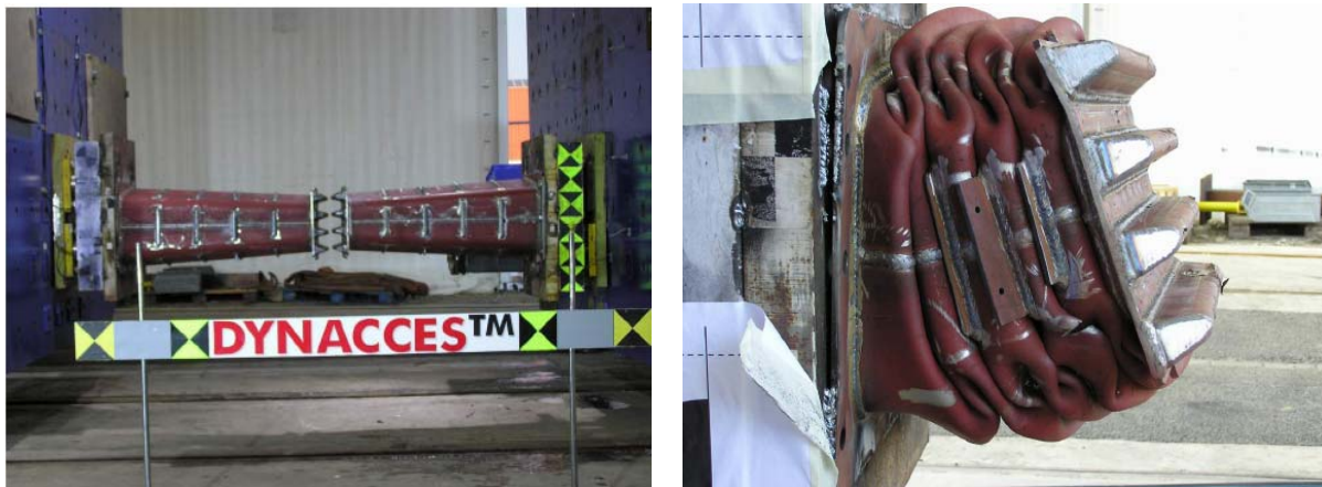
Figure 25 - Typical Cab Energy Absorber Test Results (Courtesy Alstom)
