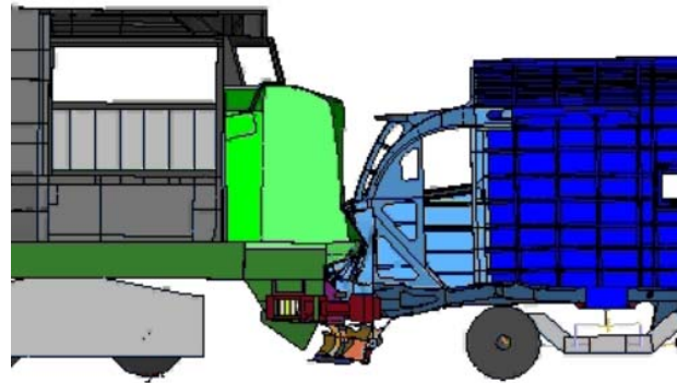
Siemens Desiro EMU-to-Locomotive Collision
