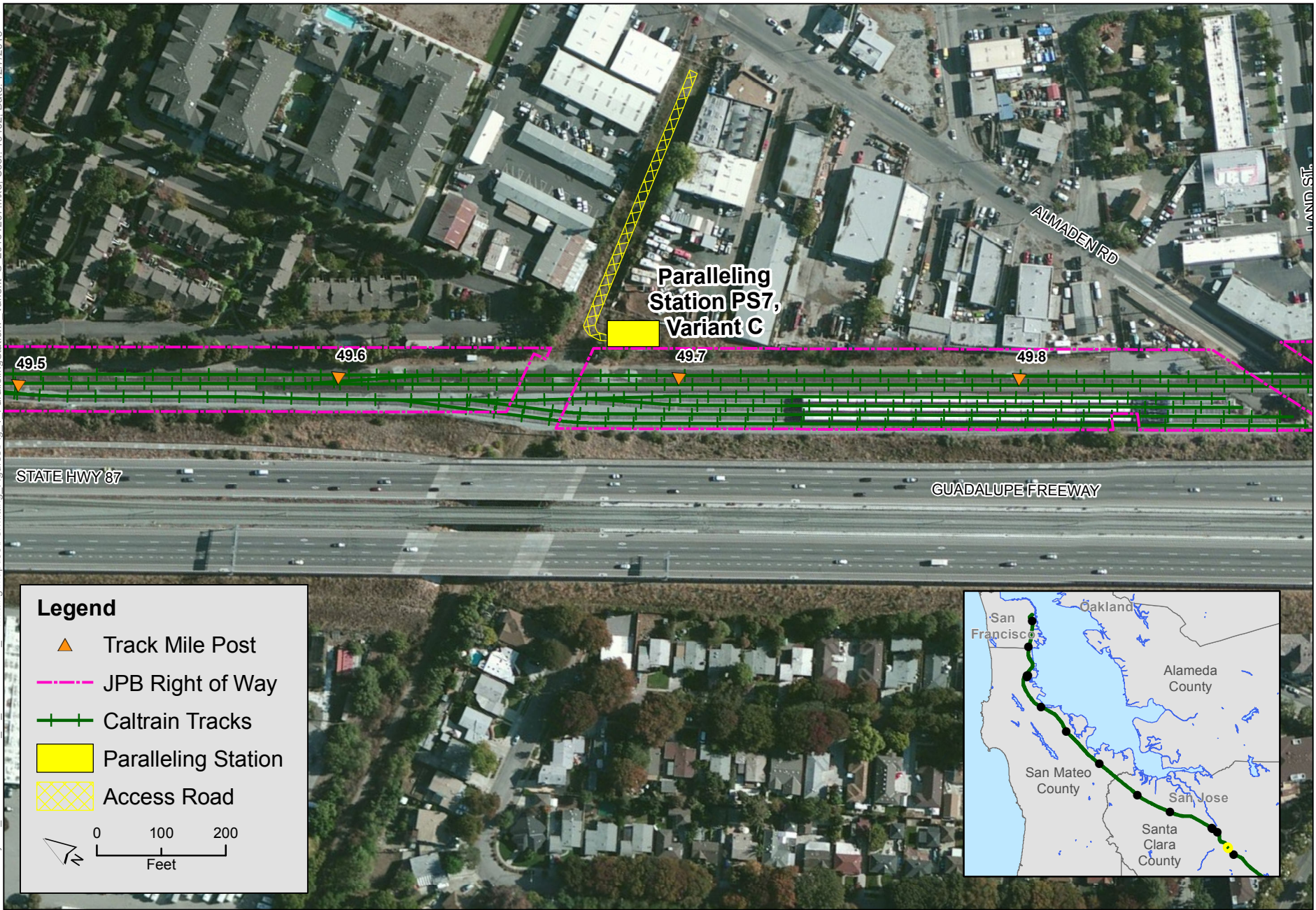
Figure 1 Proposed Paralleling Station 7 (PS 7), San Jose Peninsula Corridor Electrification Project
