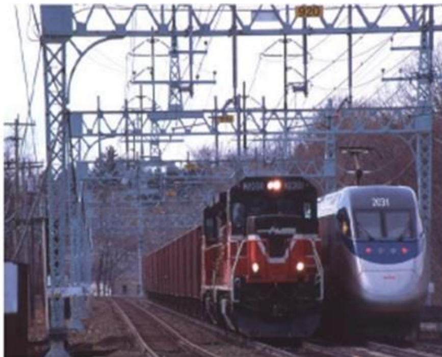
Low speed freight trains and high-speed passenger trains operating at up to 150 mph share the NEC right-of-way as illustrated here by Amtrak Acela Express operating with Providence & Worcester.
