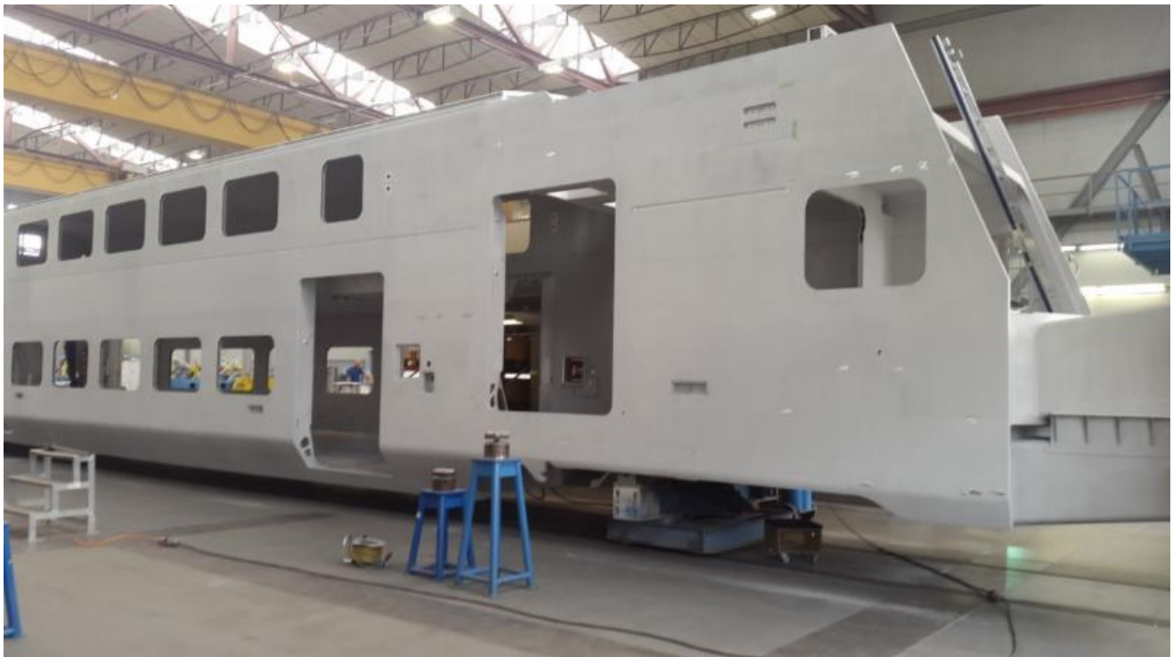
Car Shell after aluminum particles blasting
